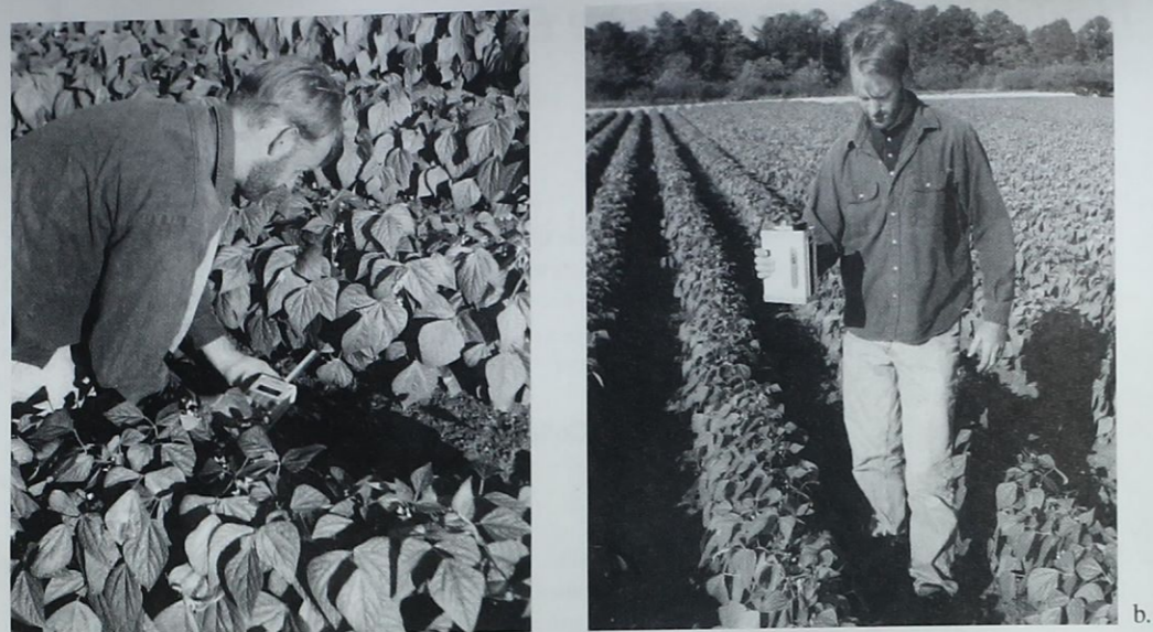
Figure 1-1 In situ (in-place) data are collected in the field at the study site. a) A scientist is collecting leaf-area-index (LAI) measurements of soybeans ( Glycine max L. Merrill ) using a ceptometer that measures the number of “sunflecks” that pass through the vegetation canopy. The measurements are typically made above the canopy and on the ground below the canopy. The in situ LAI measurements may be used to calibrate LAI estimates derived from remote sensor data. b) Spectral reflectance measurements from the vegetation canopy are being collected using a spectroradiometer located 1 m above the canopy. The in situ spectral reflectance measurements may be used to calibrate the spectral reflectance measurements obtained from a remote sensing system onboard an aircraft or satellite.
