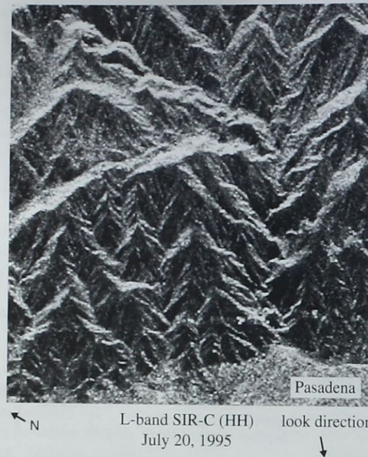
Figure 9-14 L-band SIR-C (HH) image of the San Gabriel Mountains and a portion of the city of Pasadena. Extensive layover is found in the mountainous terrain, causing the ridge lines to be displaced toward the antenna (courtesy NASA Jet Propulsion Lab).
